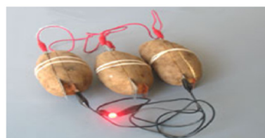
Figure 1: Series connection in lighting the LED
