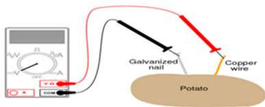
Figure 2: Diagram showing the Measurement of the Voltage Generated
