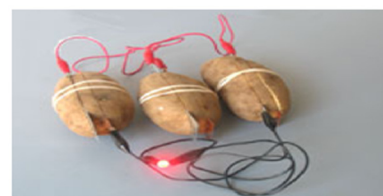
Figure 1: Series connection in lighting the LED
